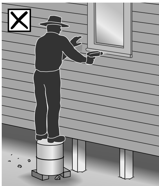
Figure 28 Hazard: makeshift means of gaining height. A safer alternative: trestles as shown in Figure 26 (b)
