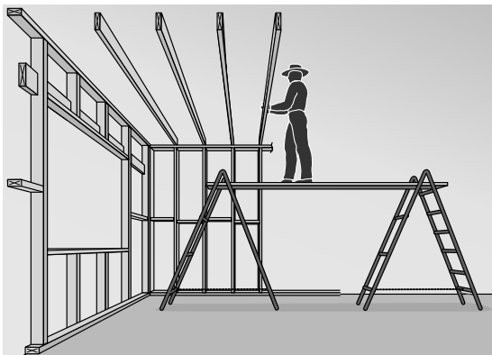
Figure 13 Installing ceiling or upper level floor joists
