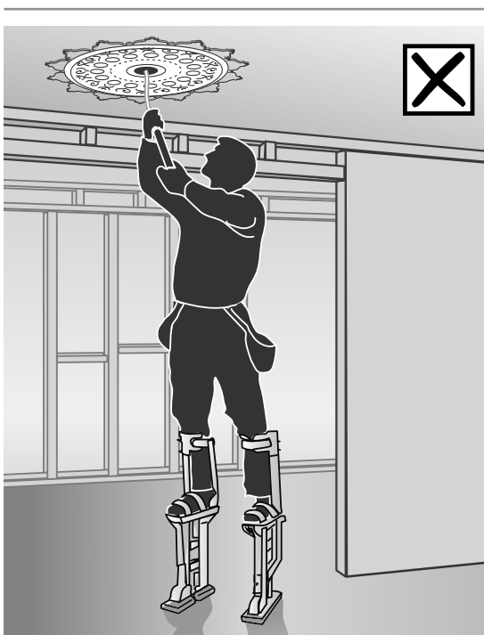
Figure 26 (a) Hazard: plasterers' stilts
