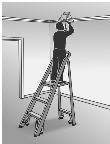
Figure 27 (b) A safer alternative: select the right ladder or step platform for the job
