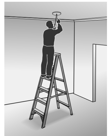
Figure 27 (b) A safer alternative: select the right ladder or step platform for the job
