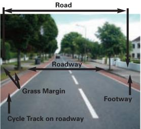
**Photograph 4** Suburban street, showing road, roadway, cycle track on roadway, grass margins and footways.
